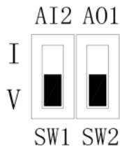
Fig.3-27 NE200 DIP switch setting
